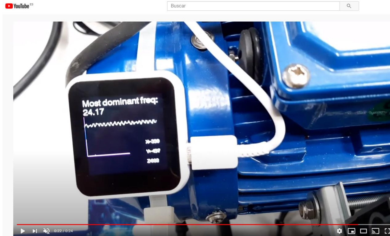
Fast Fourier Transform for predictive maintenance on electrical motors and machines
